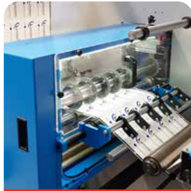
Automatic Slitting System
