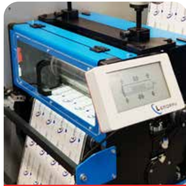
Anvil Roll with electronic adjustable gap
